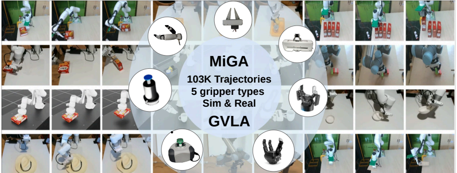
Fig. 1: We tackle the challenge of gripper-specific grasping in robotics, e.g., a suction cup gripper lifts a thin, flat, DVD-case-like box from above, while a parallel-jaw gripper pushes it to the table edge and grasps it from the side. We first introduce MiGA, a large-scale multi-gripper-aware dataset collected by diverse gripper types. Leveraging this dataset, we then develop a Gripper-aware Vision Language Action (GVLA) model that incorporates gripper conditioning through a new multi-gripper tokenization method and a dual Mixture-of-Adapter. Our approach improves task performance over gripper-agnostic baselines and enables cross-gripper adaptation.
